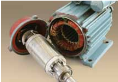
Rotor and stator of an induction motor.
