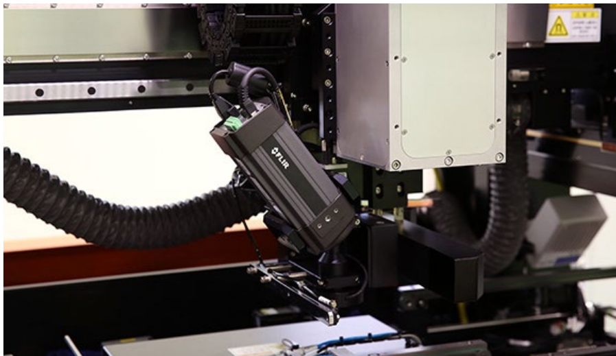
Figure 10: Cartesian robotics can be fitted with imaging equipment (such as this thermal-imaging camera) for thermography of PCBs produced with laser-assisted bonding techniques. (Image source: Teledyne FLIR )
