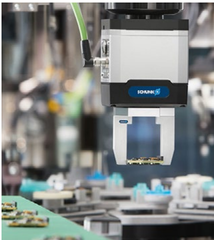
Figure 4: Small-component EGK grippers are lubricated with H1 grease and sport cleanroom certification. (Image source: SCHUNK Intec Inc. )
