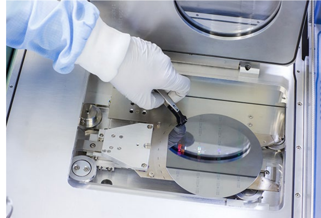
Figure 1: Here, a delicate wafer is placed into an atomic layer deposition machine located within a cleanroom. (Image source: Dreamstime)
