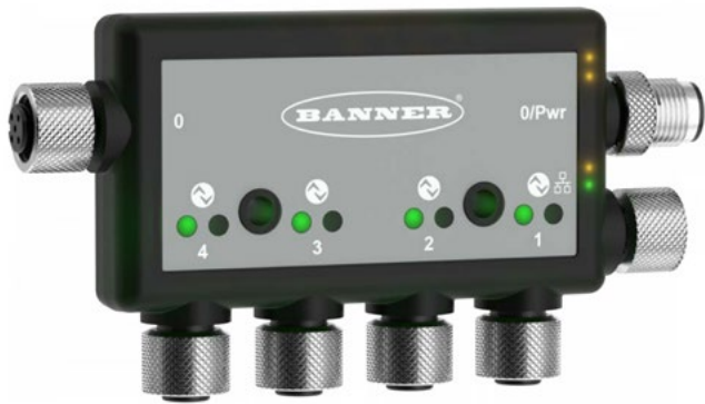
Figure 3: The DXMR90-4K IO-Link master device can combine data from four local sources and connect with a higher-level network. (Image source: Banner Engineering)
