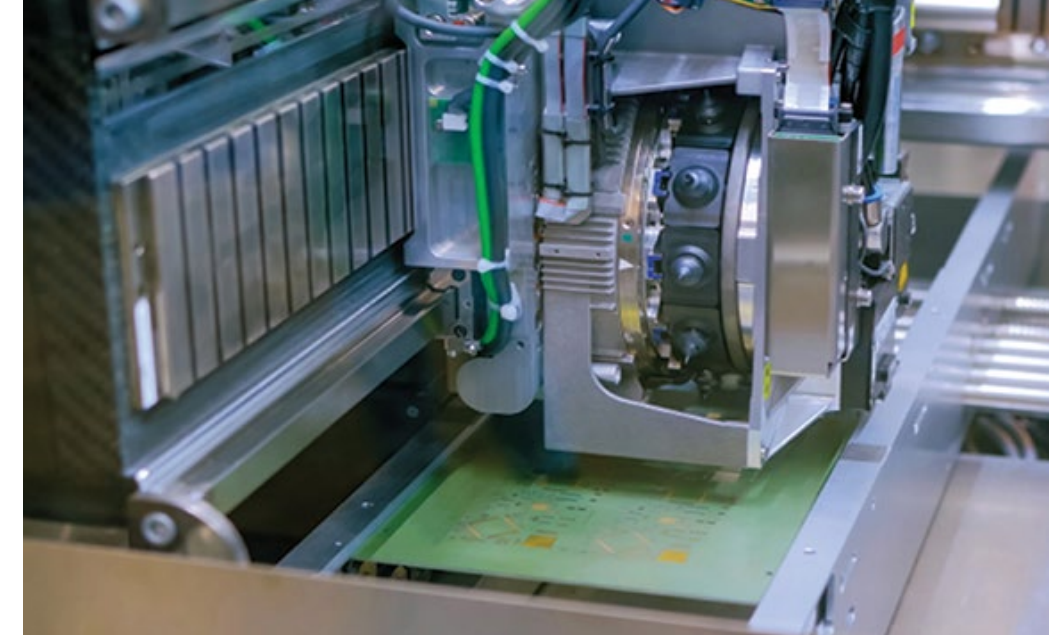
Figure 9: Cartesian robots execute fully automated semiconductor manufacturing tasks. Note the linear motors that provide high-precision direct driving on the critical axis. (Image source: Dreamstime)
