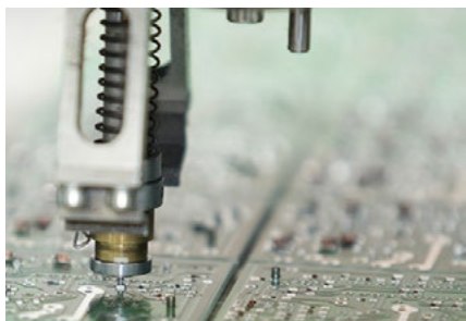
Figures 11a and 11b: Shown here are tool heads for affixing surface-mount technology (SMT) subcomponents to a board. (Image source: Dreamstime )
