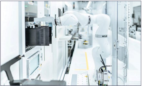
Figure 14: KUKA collaborative robots (cobots) are core to the design of this Infineon ISO3 wafer-processing cleanroom. (Image source: KUKA )
