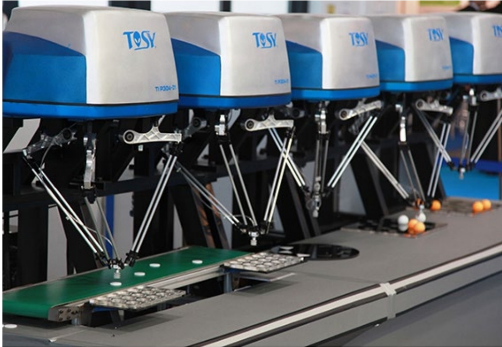
Figure 2: A delta robot is a type of parallel manipulator with three parallelograms all connected to a single rigid body at the end effector end. The base of each parallelogram is actuated in a single degree of freedom relative to the robot's base. Delta robots are typically ceiling mounted to tend conveyors or workpieces from above. (Image source: Wikimedia Commons)
