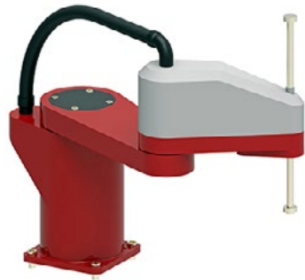
Figure 7: SCARA robots execute pick-and-place wafer handling and processing tasks quickly and precisely. (Image source: Dreamstime)
