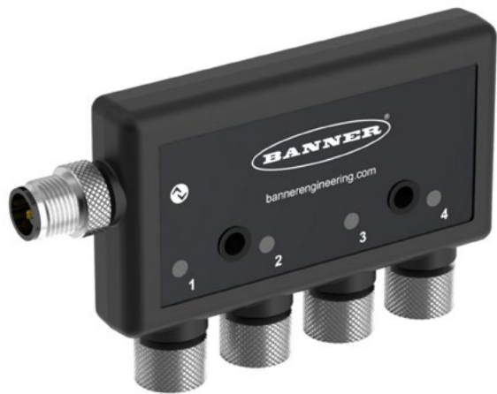
Figure 4: The R90C-4B21-KQ hub can consolidate communications from four devices and connect them with an IO-Link master device. (Image source: Banner Engineering)
