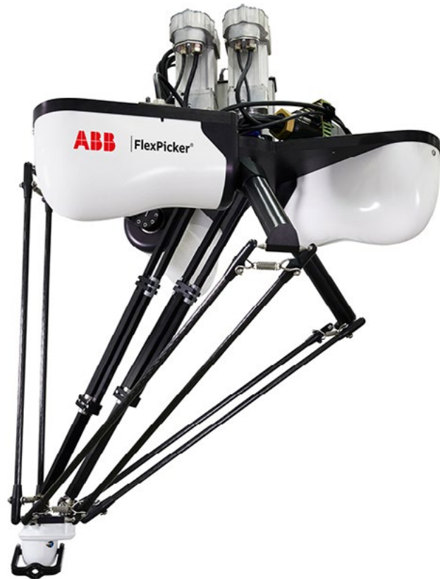
Figure 6: Some delta robots maneuver through five axes to orient objects of all types. The IRB 365 shown here can sort, feed, pick, reorient, and place 1-kg products at 120 picks per minute — satisfying the requirements of production facilities needing high throughput and efficiency. Commanded by a compact delta-robot controller called the OmniCore, the system offers performance motion control, digital connectivity, and more than a thousand programmed functions. (Image source: ABB)
