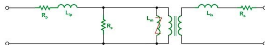
Figure 2: This basic model of a transformer shows there is no current path from primary side to secondary side.
