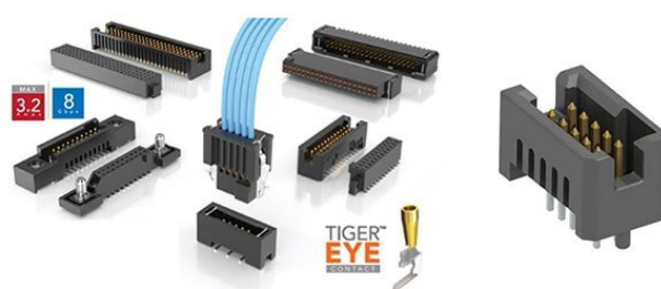
Figure 3: Tiger Eye interconnects (left) are available in a variety of formats and sizes and provide a rugged contact system rated to 10,000+ mating cycles. The TFM-105-01-S-D-A (right) is a 10-position header with 1.27mm pitch contacts.
