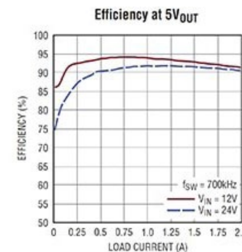
Figure 2: The highly efficient LT8620 step-down switching regulator includes a SYNC pin so its clocking can be synchronized with other system clocks, minimizing clock intermodulation effects. Image source: Analog Devices
