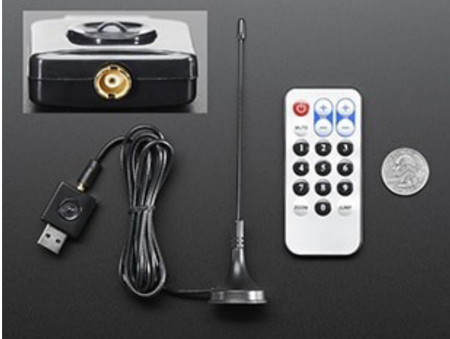
Figure 2: The 1497 is a low-cost SDR receiver that fits in a package the size of a quarter and comes with an accessory antenna and remote control. This receiver tunes from 24 MHz to 1.85 GHz, interfacing with a host computer via USB. Image source: Adafruit Industries
