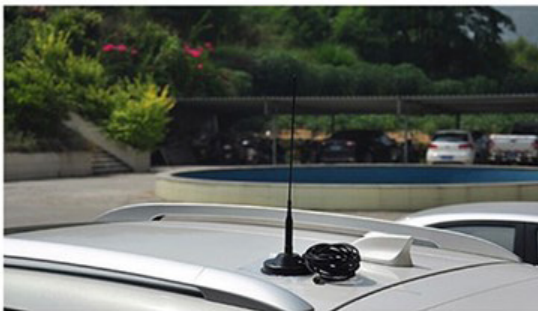
Figure 1: The long wire or whip antenna arrangement is a single-element design using a ground plane (here, the car's surface) (left); the illustration shows its simplicity (right). Image sources: Lihong Electronic (left); Electronics Notes (right)
