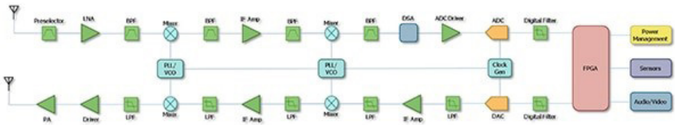
Figure 1: Traditional superheterodyne radio architectures can meet performance targets, but their complexity prevents them from meeting emerging targets for minimal SWaP. Image source: Analog Devices
