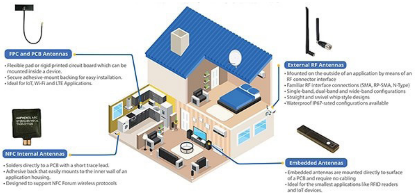
Figure 4: Different antennas are available to suit various IoT applications. Image source: Amphenol
