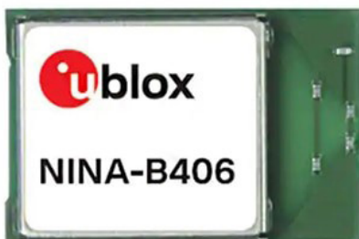
Figure 6: AoA and AoD applications that benefit from an integrated antenna can use the NINA-B40x series modules.
