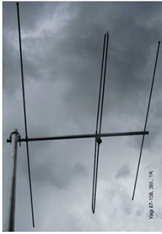
Figure 3: The basic Yagi antenna (top) is a three-element antenna widely used in commercial, residential, and military applications. The three elements (bottom) are a driven (active) dipole element with a passive reflector behind it and a passive director in front of it, all mounted on a single boom. Image sources: EuroCaster/Denmark (top); RFWireless-World (bottom)
