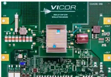
Figure 6: The DCM3623EA5N53B4T70 evaluation board enables designers to explore the capabilities of the DCM3623TA5N53B4T70 DC/DC converter. Image source: Vicor
