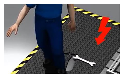
Figure 1: Safety mat operation requires physical contact and can be compromised by accidents and environmental hazards. (Image source: SICK)
