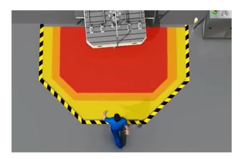
Figure 3: ISO 13855 guidelines can be used to calculate the sizes of safety fields (red) for safety laser scanners like the S300 Mini Standard. (Image source: SICK)
