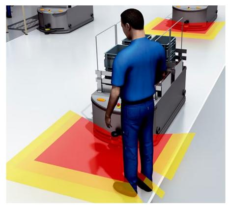
Figure 4: The compact size of S300 Mini Standard safety laser scanners enables them to be mounted on small AGVs. (Image source: SICK)
