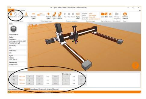
Figure 2: The "Jogging" tab (bottom left) in the iguverse immersive development environment can be used to enter motion profiles. (Image source: Igus)
