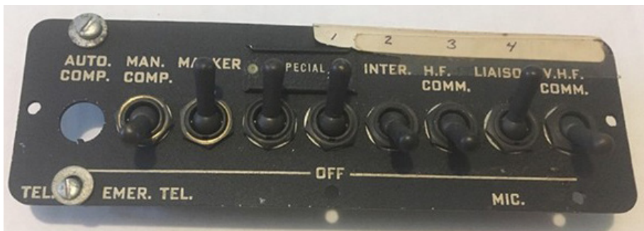
Figure 6: This array of military surplus toggle switches was used to simulate the action of limit switches on a load frame during an ongoing product development process. Image source: Bill Schweber
