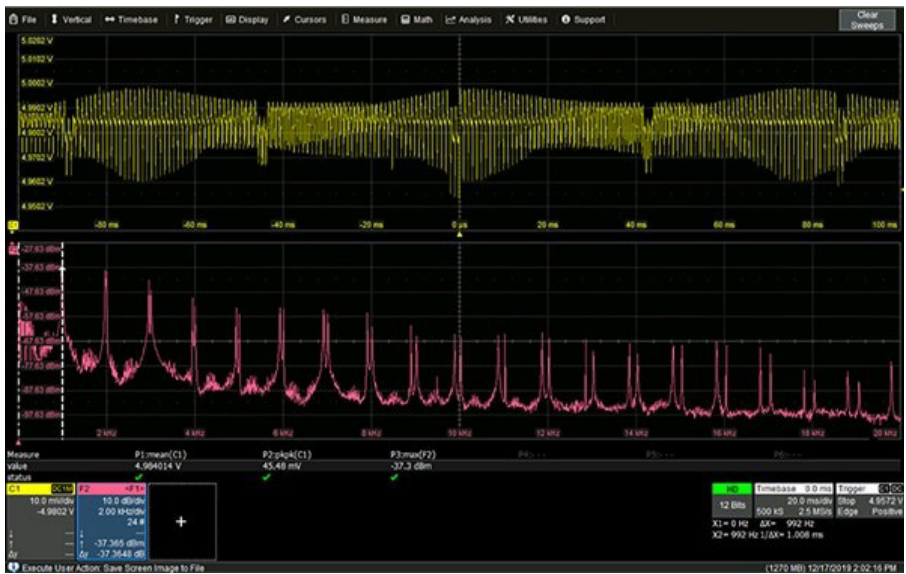
Figure 3: A power integrity measurement on a 5 volt bus for a daughter card shows the ripple voltage and the FFT of the ripple. Image source: DigiKey
