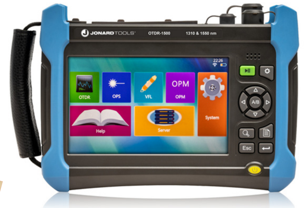
Figure 1: The Jonard Tools OTDR-1500 Image source: Jonard Tools
