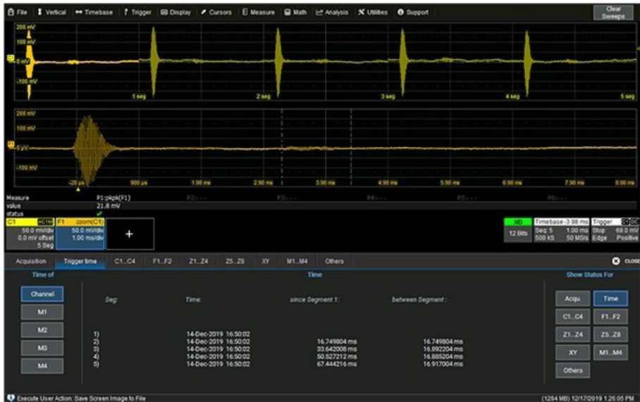
Figure 2: A Teledyne LeCroy WaveSurfer 4104HD oscilloscope used in the acquisition of a 40 kilohertz (kHz) ultrasonic range finder signal. At top it shows five pulses for each measurement spaced about 16.8 milliseconds (ms) apart.
