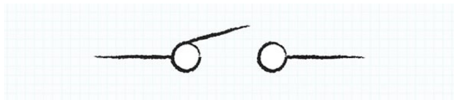
Figure 1: SPST switch diagram. (Image source: Same Sky )
