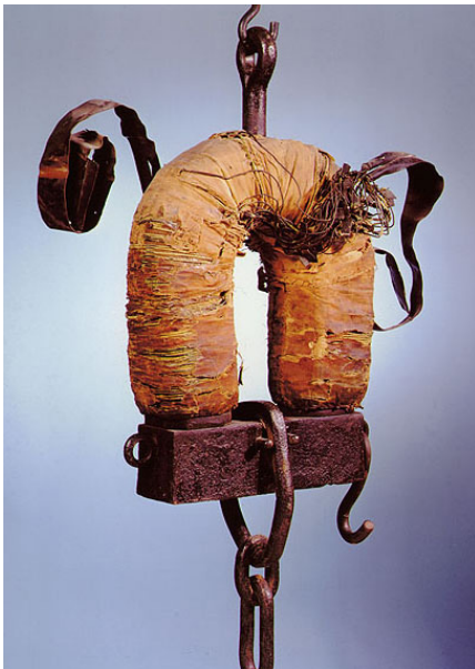
Joseph Henry’s large electromagnet built for Yale College.
