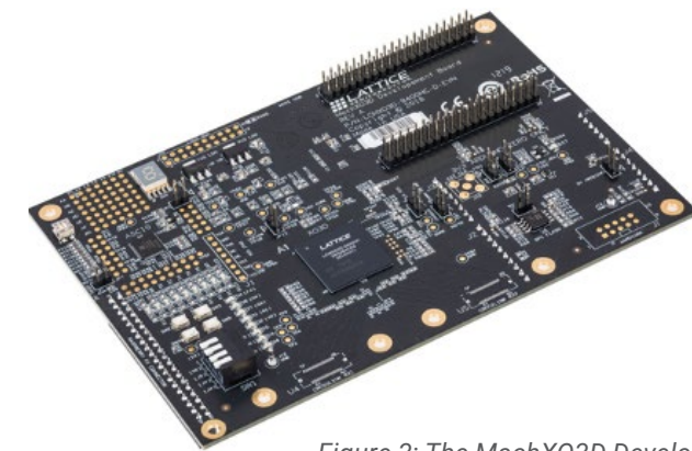
Figure 3: The MachXO3D Development Board features a MachXO3D FPGA, an L-ASC10 (analog sense and control) hardware management device, support for Arduino and Raspberry Pi boards, two Hirose FX12-40 header positions (DNI), an Aardvark header, and a USB-B connection for device programming. (Image source: Lattice Semiconductor)
