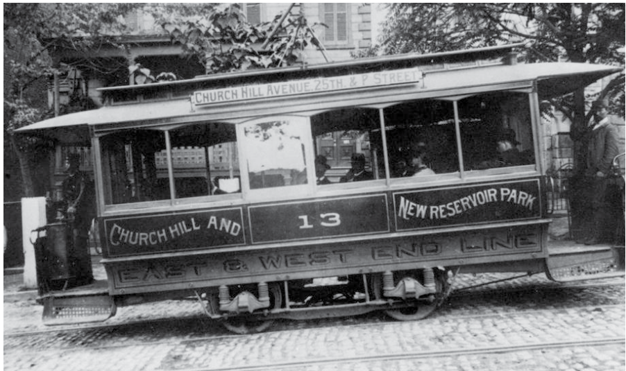
Sprague's unique undercarriage motors made the steep inclines a trivial task.
