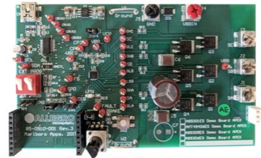
Figure 5: The APEK89307KET-01-T-DK eval board has the A89307KETSR-J (U1, center left hand side of the board) and six power MOSFETs (right hand side) to drive a BLDC motor. (Image source: Allegro MicroSystems)
