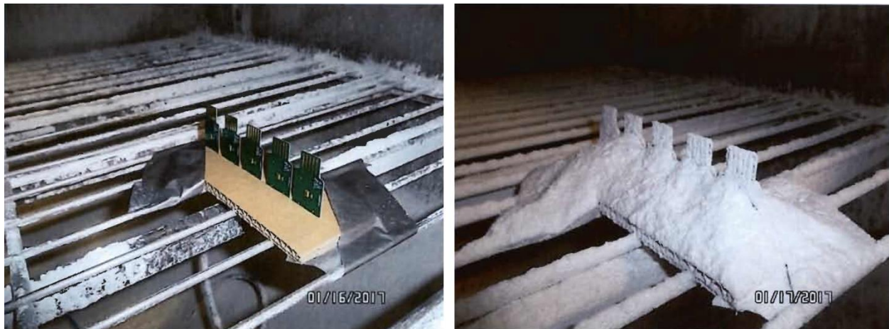
Figure 13: Vesper piezoelectric MEMS microphones mounted on test boards, before (left) and after (right) and IP5X dust test
