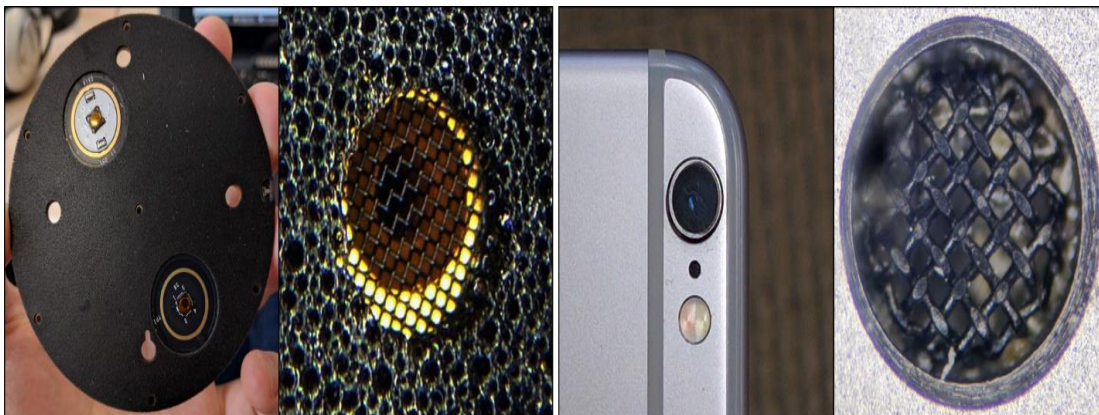
Figure 4: Amazon Echo microphone array & zoom-in of microphone mesh (left), iPhone 6S rear microphone & zoom-in of microphone mesh (right)
