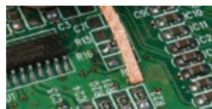
Match braid width to contact area
