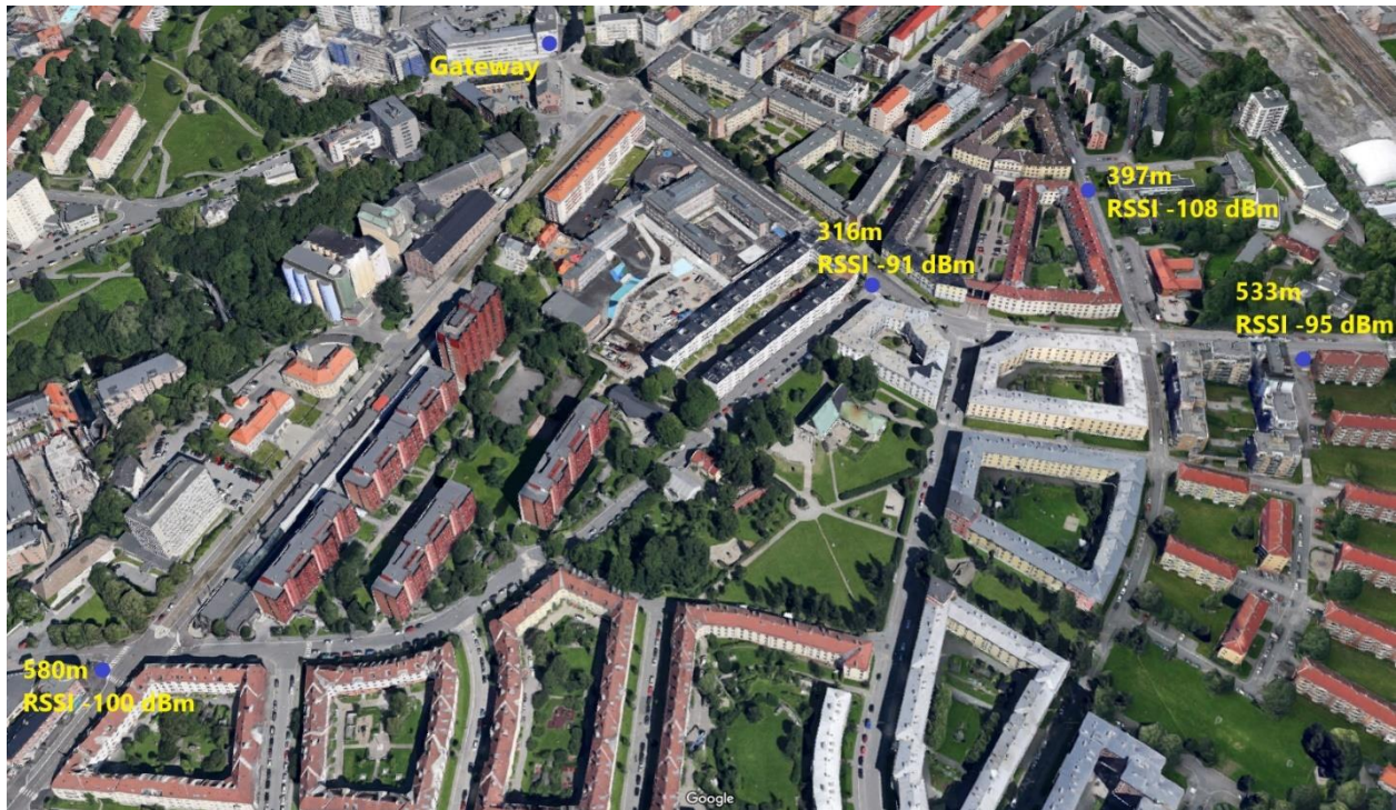
Figure 9. Coverage map around Radiocraft's office in Oslo city for 5 kbps mode.
