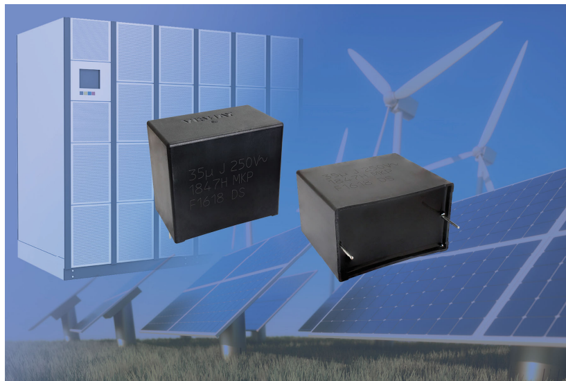
Figure 1. The devices shown here (MKP1847H) are the industry's first full-range AC filtering film capacitors to withstand demanding temperature humidity bias (THB) testing — 85 °C, 85 % RH for 1,000 hours at rated voltage — without altering their electrical characteristics. The capacitors feature segmented film and offer rated capacitance from 1 \mu F to 35 \mu F and low ESR down to 3 m \Omega . The devices provide high ripple
