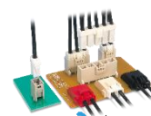
DF22 Rated Current : 30A Max. Rated Voltage : 1000V AC/DC Pitch : 7.92mm No. of Pos. : 1-5 AWG : 10-16
