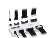
DF50/DF50A Rated Current : 1A Max. Rated Voltage : 100V AC/DC Pitch : 1.0mm No. of Pos. : 20, 30, 40, 50 (DF50) 2-16 (DF50A) AWG : 26-32
