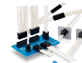
DF63 Rated Current : 15A Max. Rated Voltage : 630V AC/DC Pitch : 3.96mm No. of Pos. : 1-6 AWG : 16-22
