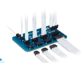
KW30 Rated Current : 1A Max. Rated Voltage : 100V AC/DC Pitch : 1.0mm No. of Pos. : 30 AWG : 28-32
