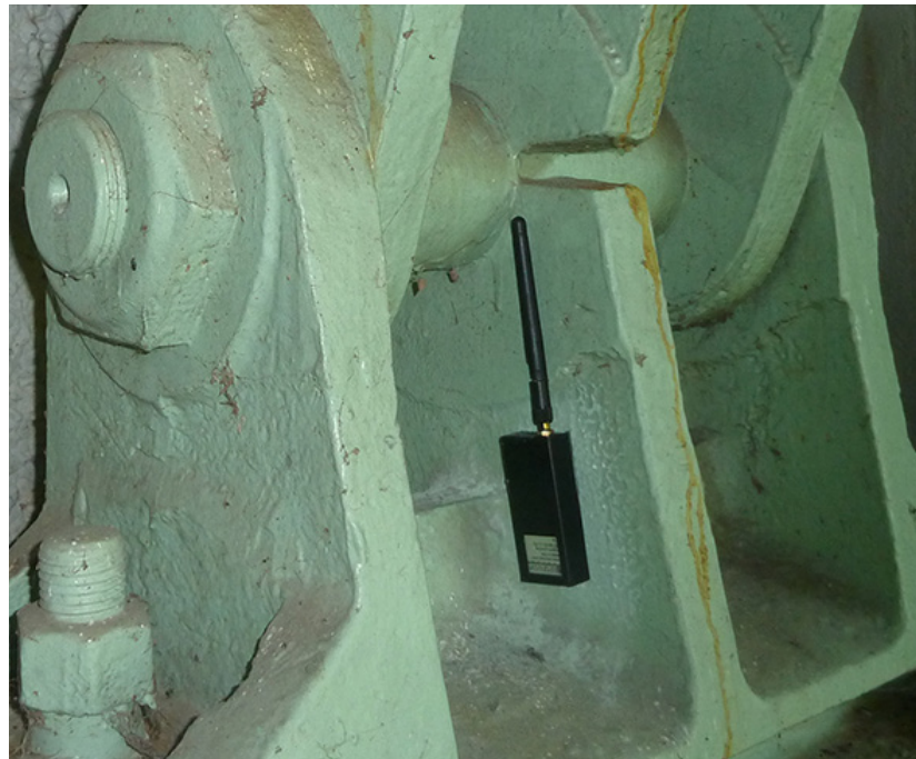
Resensys structural stress monitors are mounted beneath bridge trusses and other hard-to-access locations. These monitors require ultra-long-life bobbin-type \text{LiSOCl}_2 batteries to minimize the need for costly and dangerous battery replacements.
